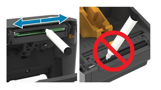
Clean printhead with a cleaning pen. Clean from the middle to the outside. Do not use a cleaning pen on the platen.
