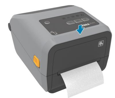
Press down on the front edge of the printer until it locks.
