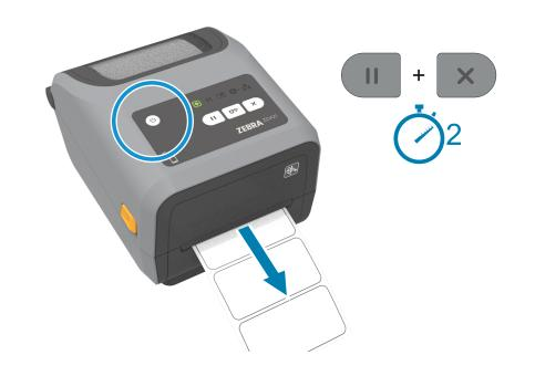
Press and hold the Pause and Cancel buttons for two seconds to line up the labels.
