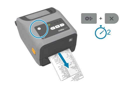
Press and hold the Feed and Cancel buttons for two seconds to print a configuration report.
